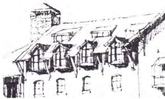
Fig 8-27: Dormers can lend “texture” to the overall roofscape of Lionshead.
