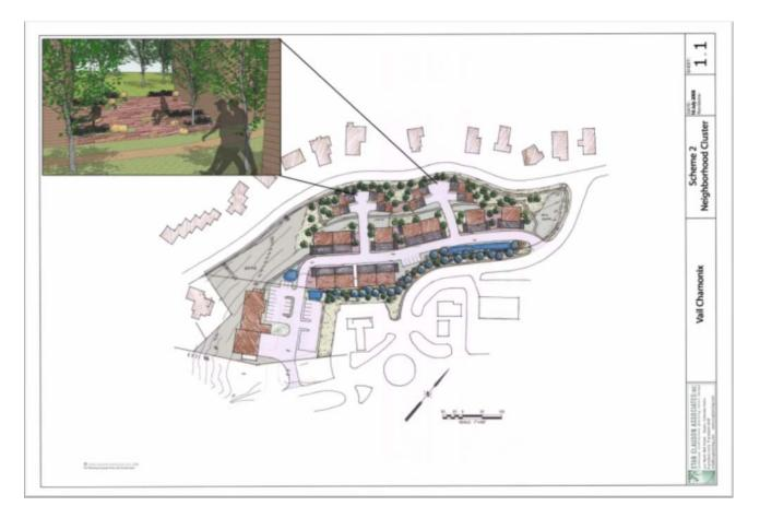
The unit mix provided for 68,232 sq. ft. of housing with a density of 14 dwelling units per acre. A main access street, which gained access to the site from Chamonix Road, passed through the site to the fire station, again offering dual points of access. Access to the fire station was limited for safety reasons. Multi-family units were situated off the north and south side of the access road. Drives extend to the north off the main street to duplex units.
