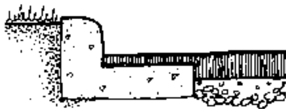
CONCRETE CURB AND GUTTER WITH ASPHALT OVERLAY
